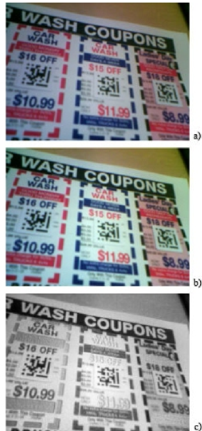
Fig. 4 a) Original Image, b) Image after Scale By Max Applied and c)Image after gray scaling
