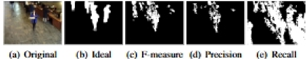
Fig. 1. Results of maximizing the F-measure (c), precision (d), and recall (e) on the B sequence in the Wallflower data-set. This sequence has foreground objects present during the background subtraction initialization, and as such it tests how quickly a background subtraction algorithm can learn the true background and let the false background become foreground.
