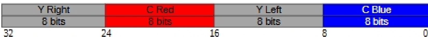
Figure 1: Pixel Pair Representation (Y is luminance, left and right is the pixel in the pair)
