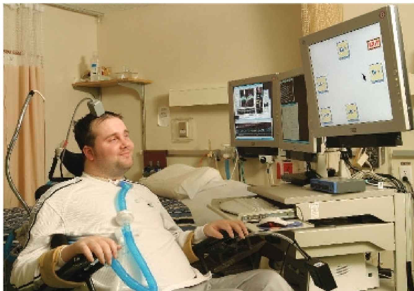
Mind control: Matt Nagle's neuroprosthetic lets him move a cursor using thought alone.
