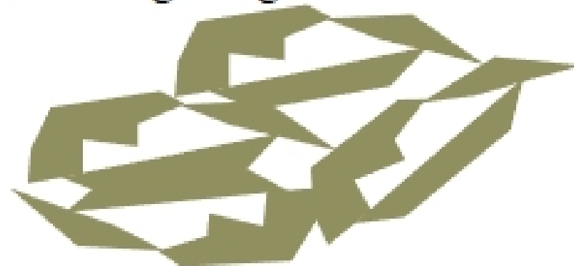
Loose, angular soil
