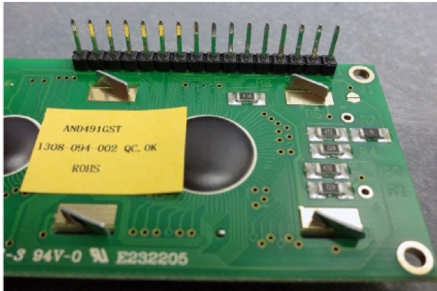
Figure 2: LCD module with connector.
