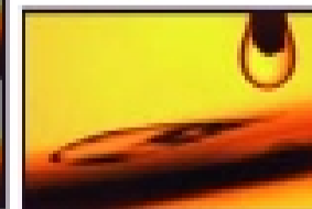
Figure 3. Microscope image of a superfluid drop on a Cs substrate inclined at 10° to the horizontal. A drop hanging off of the capillary is also seen in the upper right. The drop on the inclined substrate is stationary. The downhill edge of the drop has the same contact angle as shown in Fig. 2B, whereas the uphill edge has a vanishing contact angle.
