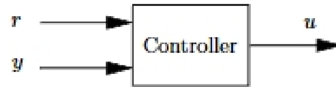
Figure 10.1: An abstract representation of a controller with two degrees of freedom.
