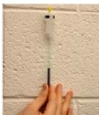
Spinner on an NMR tube. The placement is too high. No signal would be seen.
