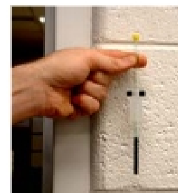
Approximate height of spinner on an NMR tube. Note that the person is not touching the spinner.
